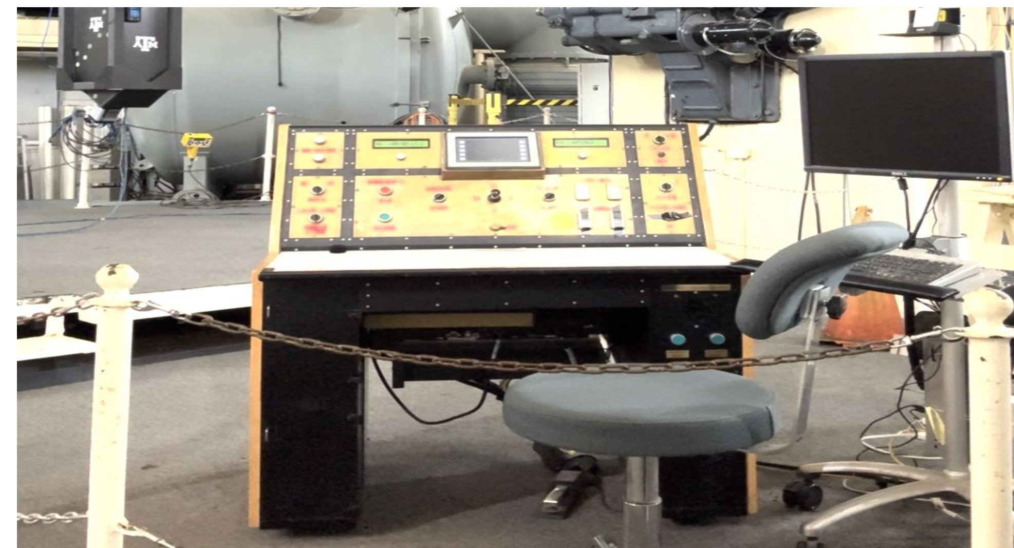
Figure 2. Otto Struve 82" telescope Control System
