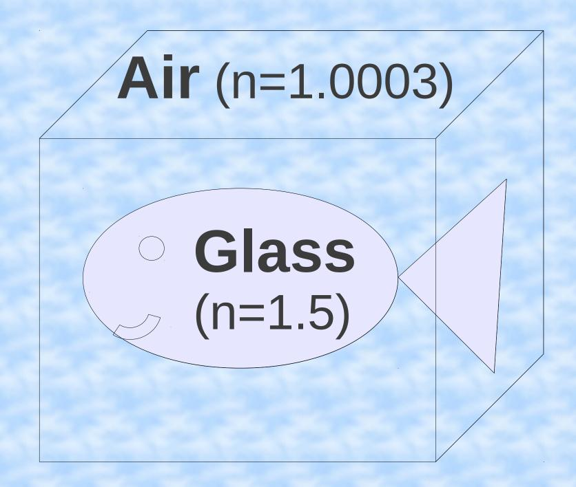
That is why we can see the clear glass fish in the clear air! Glass, air, and water each bend light in different amounts. They have different index of refraction (n).
